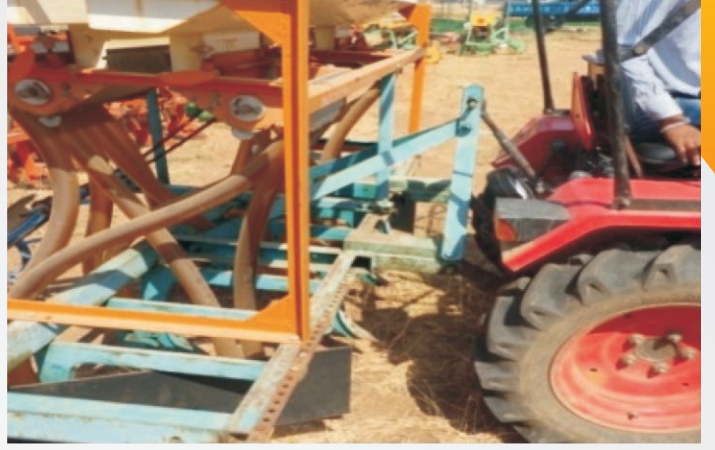
Mini tractor with modular maize planter and Seed cum fertilizer drill (Khedut)
